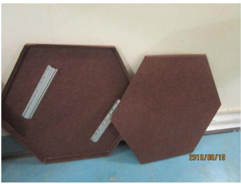
Figure 3 – Body and lid pieces, metal rails at body interior
