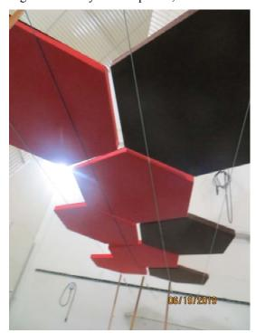
Figure 4 – Underside of installed specimen, spacing between units
